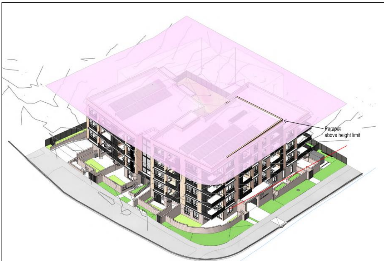
Figure 2 – Building height plane showing parapet protrusion (Source: Morson Group)
